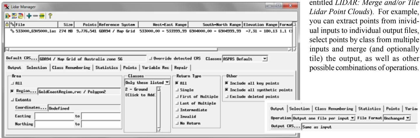
The Selection panel provides controls for choosing points for extraction by area, by class, and by return type. The extraction area can be limited using a region object (as in the illustrated example) or by specifying rectangular extents in any coordinate reference system. The Classes controls allow you to create a list of classes to
