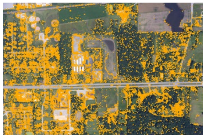
Vector points (orange) showing locations of over 125,000 keypoints (AKAZE detector) for a lens-corrected aerial camera image.
