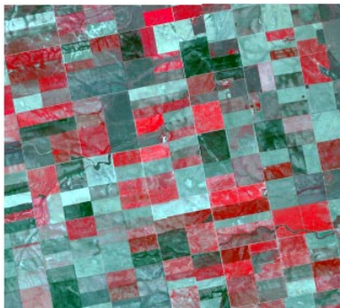
Color-infrared display (Display Red = NIR, Green = Red, Blue = Green) of agricultural fields with various states of crop cover. Red areas correspond to dense crop cover.
