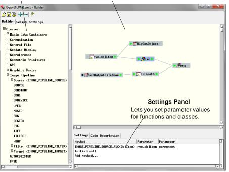
connections are shown by the gray lines in the design canvas, and the component inputs and outputs are represented by arrowheads in the boxes. Connecting components establishes a sequence of execution and automatically generates SML code that can be viewed and run at any time using the Script tabbed panel. Script designs can be saved to, and reloaded from, a file (\*.smlb) that stores your selection of script components and their settings, positioning in the design space, and connections.
