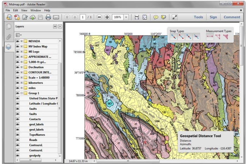
PDF file rendered from a complex TNTgis map layout with layer controls included, so any individual layer can be toggled on and off in Adobe Reader. Georeference information is automatically transferred to create a Geospatial PDF file. Adobe Reader provides a Geospatial Location Tool to provide coordinate readouts (in Latitude/Longitude) and a Measuring Tool (shown above) to measure distance, perimeter, and area (tools available on the Edit / Analysis submenu in Adobe Reader XI).
