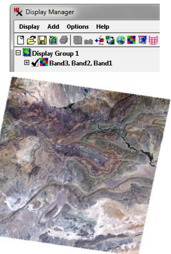
Result from Add as RGB raster layer: fixed color display using the specified 3 bands.
