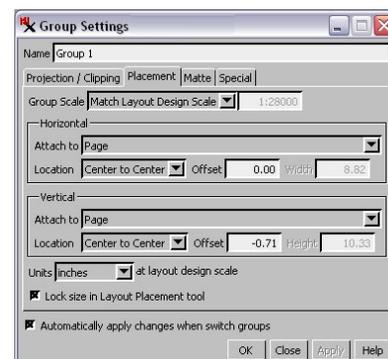
The Placement panel lets you set the group(s) to which horizontal and vertical attachments are made and the spacing (Offset) from them. The Placement panel is active for groups that are not auto-matched to another group.
