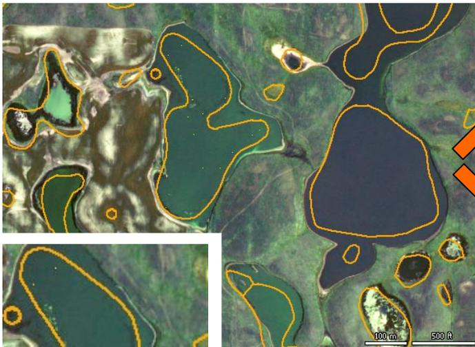
Natural-color orthoimage with a number of ponds with differing depths and water color. Reference vector polygons are shown with the orange outlines. The Define Samples tool was used to identify a number of sample cells within one pond polygon (enlarged at left).
