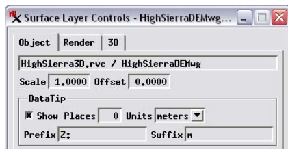
You can set vertical Scale and Offset values for stereoscopic and perspective renderings on the Object tabbed panel in the Surface Layer Controls window.
