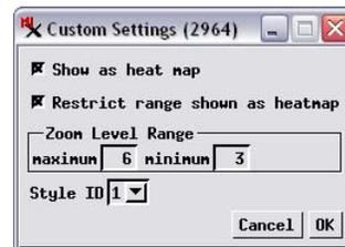
The Custom Settings dialog for a Fusion Tables layer lets you choose to display the data as a heat map for a specified range of layers and use the normal map styling for the remainder of the zoom level range.
