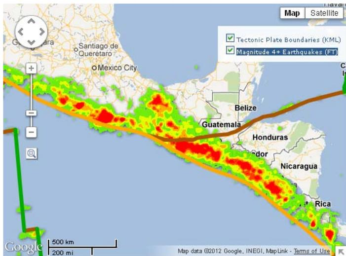
Geomashup of Central America region with a Fusion Table layer of earthquake epicenters and a KML layer showing tectonic plate boundaries (colored lines). The Fusion Table layer options were set to show a heatmap visualization of the earthquake locations from Google Maps zoom levels 3 through 6 (zoom level 5 shown above left) and the earthquake points at higher zoom levels (zoom level 7 shown above right).
