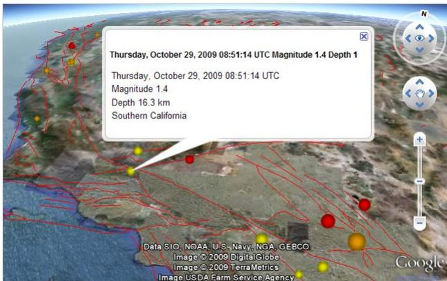
Google Earth plug-in displaying KML earthquake overlay produced by the sample script and the native Google global imagery. The feature balloon information shown when an earthquake epicenter marker is clicked is transferred to the KML file from the TNT DataTip settings.
