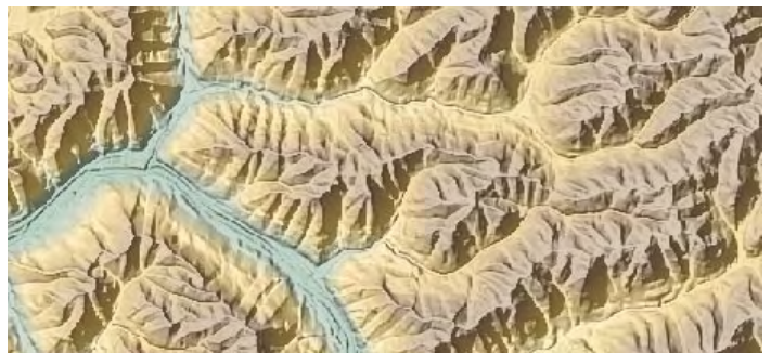
5 x 5 Volterra/Unsharp sharpening filter applied only to the shading raster layer, producing a crisper image of the terrain.
