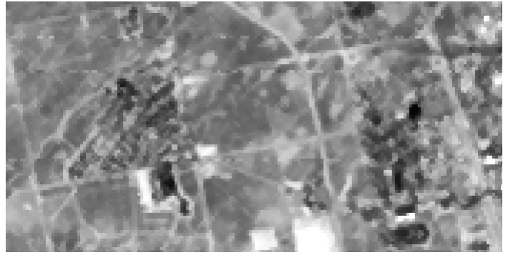
is the pure filtered image result. The scan-line noise is greatly reduced by the smoothing effects of the P-Median filter, while considerable edge and line detail is preserved along the roads and field boundaries.
