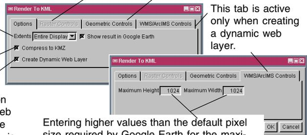
Entering higher values than the default pixel size required by Google Earth for the maximum height and width increases the resolution at various zoom levels at the expense of slower display speeds in Google Earth.
