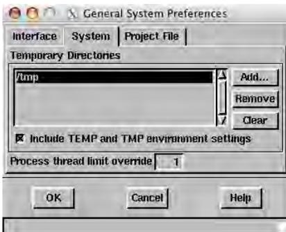
To test your multi-core system's TNT performance against a simulated single-core system, temporarily set the Process thread limit to 1 in the General System Preferences (Tools / System / Preferences). You must restart TNTmips in order for this change to take effect.
