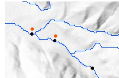
Input sample points (orange dots) may not lie exactly on the flowpaths calculated by the watershed function, so the script snaps each sample point to the closest vertex on the closest flowpath line (black dots) within the specified search distance before delineating the upstream catchments.
