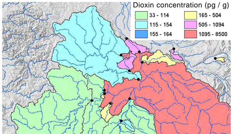
Stream sediment sampling locations (black dots) monitoring dioxin pollutant levels in the lower Willamette River basin (Oregon, USA). Upstream catchment polygons determined by the SampleCatchments script for these locations are theme-mapped by dioxin concentration (in picograms dioxin per gram of sample).
