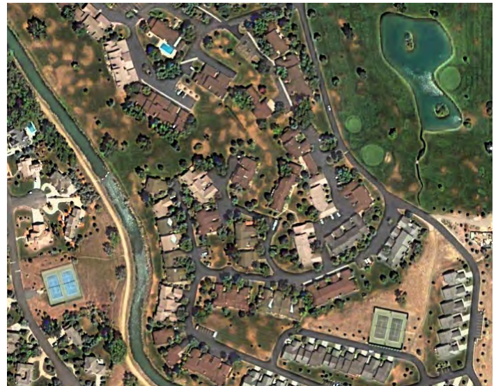
Pan-sharpened natural-color composite produced in the Multiresolution Fusion process from this QuickBird scene using the sensor-tailored calibration. The result using the Paris color fusion method is a 0.7-m color image with proper color balance.
