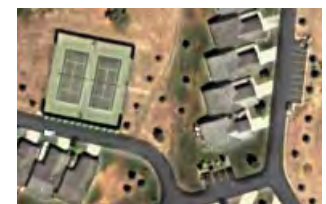
Pan-sharpened natural-color composite produced in the Multiresolution Fusion process from this QuickBird scene using the sensor-tailored calibration. The result using the Paris color fusion method is a 0.7-m color image with proper color balance.
