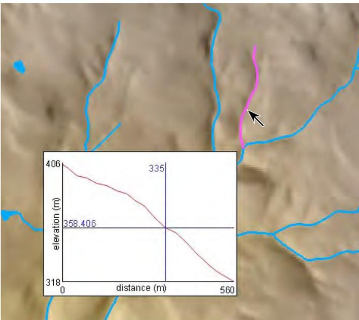
In this example the position of the GraphTip is also varied depending on the position of the cursor in the View in order to prevent it from obscuring the highlighted line element.
