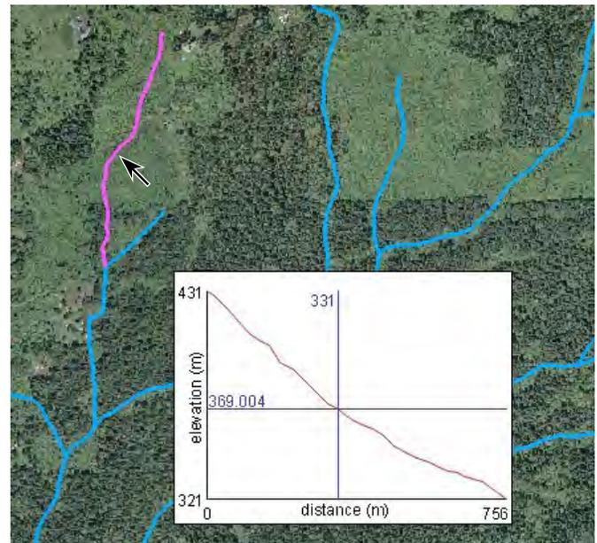
This GraphTip obtains elevation values from a raster object that is the bottom layer in the group, and highlights vector lines in the top layer in the group. Intervening layers can be turned off or on without affecting the operation of the GraphTip, as shown by the photo layer turned on in this illustration.
