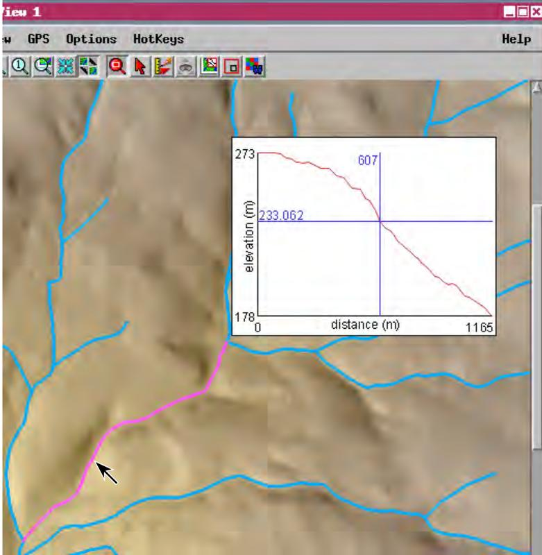
A GraphTip can include multiple graphic elements including text, with each element independently positioned. In this example the vertical and horizontal cross-hair lines indicate the position of the cursor along the line in both distance and elevation.
