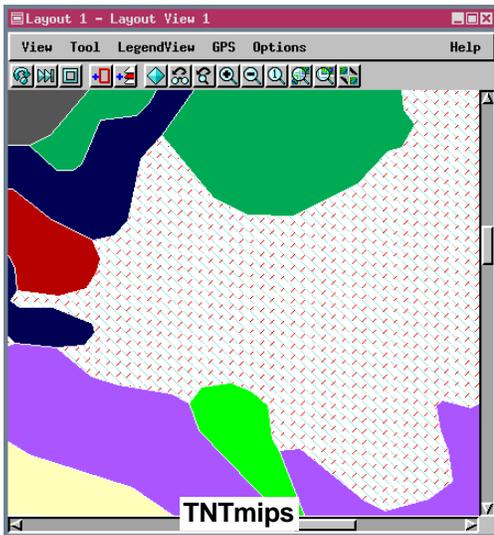
A hatch pattern in the TNT products is a fill pattern made up of lines with width that does not change as you zoom in and out. Hatch patterns used for polygon filling in your layouts can now be converted to Adobe Acrobat files (.pdf), Adobe Illustrator files (.ai), and Scalable Vector Graphics files (.svg and .svgz) by printing from the Spatial Data Display process. You select the appropriate file type from the list of printers in the Page Setup window. These graphics programs do not
