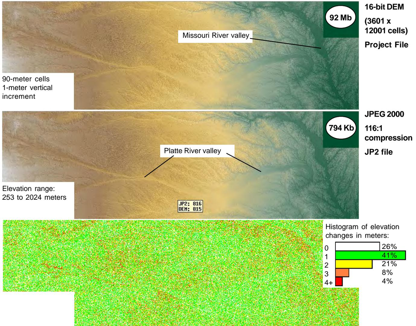
The image above is a difference raster, which shows a cell-by cell comparison of the original 92Mb 16-bit integer elevation raster and the lossy 794KB JPEG2000 compressed JP2 file.
