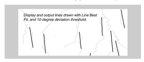
Lines selected that have an orientation of 20 degrees from North. Selection parameters allow 10 degrees of deviation, and a minimum line length of zero (0).
